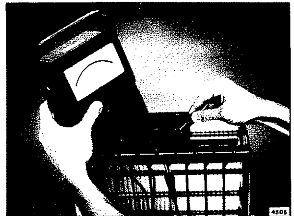
FIG. 22—USE AN OHMMETER TO CHECK THE ELECTRONIC CELLS FOR SHORT CIRCUITS.
