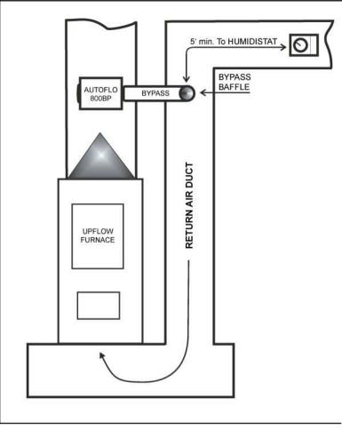
Typical field configurations for UP FLOW and HORIZONTAL FLOW furnances and air handlers. Your actual configuration may vary. Additional by-pass duct may be required, but keep the by-pass duct as short as possible. The by-pass duct should *never* be routed across the front of the furnace. All furnace access doors and openings must remain unobstructed for proper furnace operation and servicing. Remember to cap off the unused end of the humidifier.
